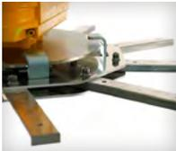
**HUB:** The fan hub shall be 19" (48 cm) in diameter and shall be made of precision-cut aluminum for high strength and light weight.
