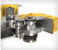
**DURABLE GEARBOX:** The NitroSeal™ drive gearbox design is lubricated for the life of the product (no oil changes required). The gearbox is equipped with a hollow shaft threaded to accept a 3/4" NPT fitting in which wiring, piping, etc., can be routed to below the fan. A standard junction box can be affixed to this hollow shaft.
