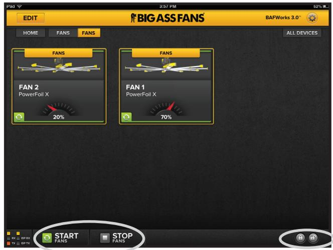
Figure 4—Starting, stopping, and locking/unlocking fan groups
