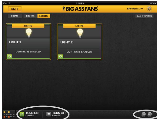
Figure 11—Turning on/off and locking/unlocking light groups
