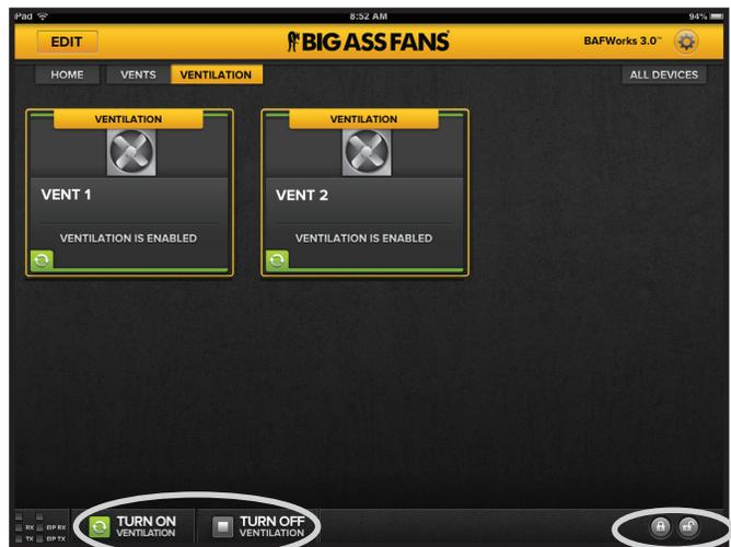
Figure 16—Starting, stopping, and locking/unlocking vent groups
