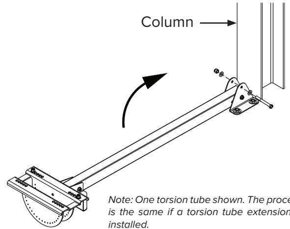
*Note: One torsion tube shown. The process is the same if a torsion tube extension is installed.*
