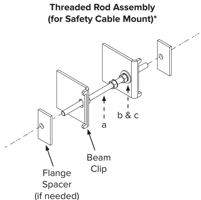
\*Beam clips and flange spacers used on the Column Mount are larger than those used on the Safety Cable Mount.
