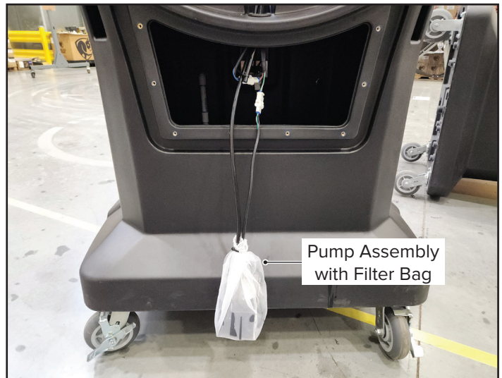
Fig. 2.2: Remove pump assembly
